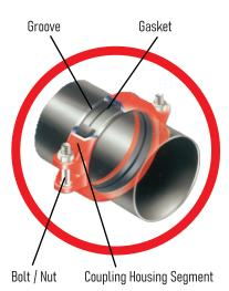
7 A flexible coupling accommodates pipe deflection and or non-alignment as below:-
