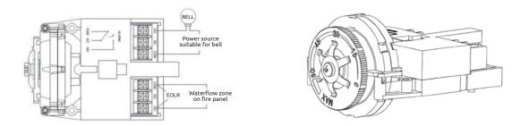
Note : Retard Structure can be set from "0" to "MAX" position, delay time can be set from 0~90 secs.
