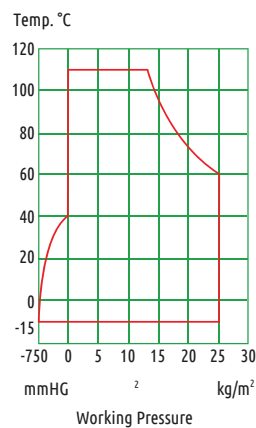
F83DJ25 DN32 ... DN200 Burst Pressure 60bar
